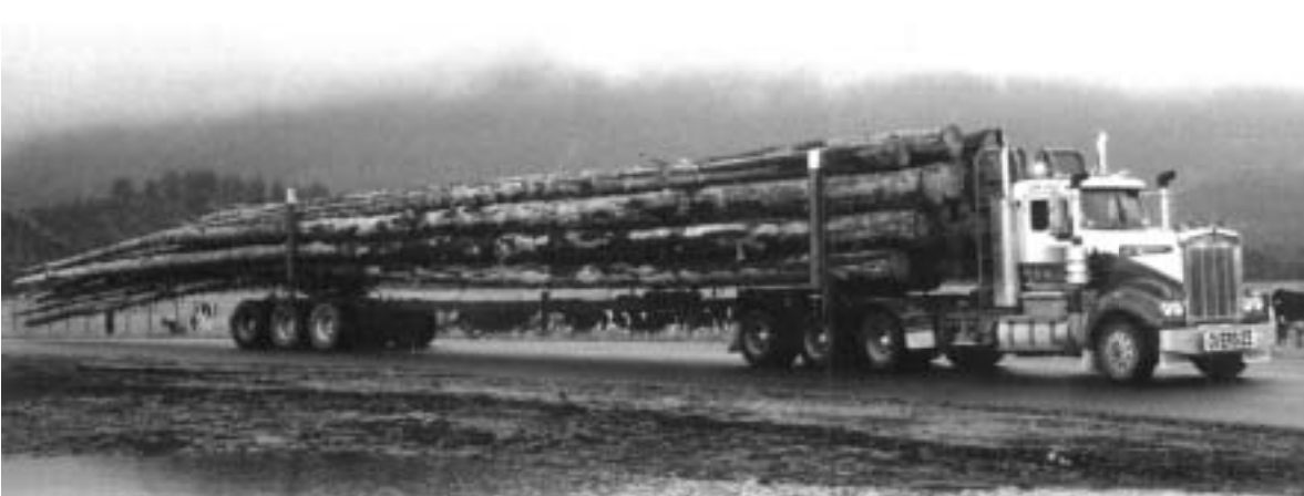
Logging truck from Kawerau - the trees on this triple-axle Kenworth were 31 metres long and the load weighed in at 109 tonnes.
