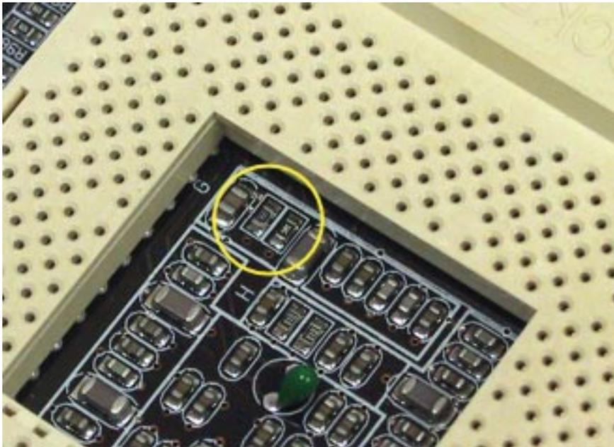
3) Find the two impedance control resistors. They are side by side, right inside the CPU socket, as shown circled in yellow.
