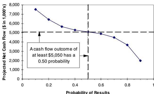
Figure 4. Sample results from Monte Carlo simulation with the financial model. The curve shows the probability that cash flow results will total at least to the level indicated on the vertical axis.
