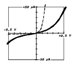
Fig. 1. Characteristic curve for the replica detector. The curve for a typical point contact germanium diode (OA81, 1N34) is shown by dotted line.
