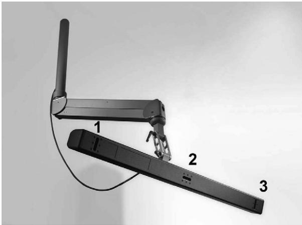
Fig. 2. Synchrony camera array has three 1-dimensional CCD cameras (1, 2, 3), which are capable of determining the positions of LED markers attached to the patient's vest at a rate of 25 to 40 Hz. Image used with permission from Accuray Incorporated.
