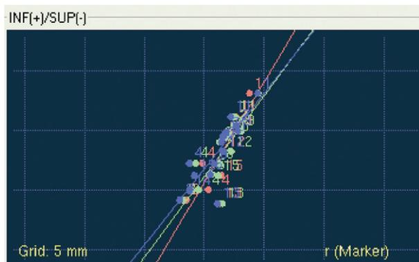
Fig. 4. A plot of internal vs. external marker position for I/S direction. Similar plots for A/P and L/R directions are also computed. Dots in the graph represent the correlation between the internal marker positions extracted from diagnostic x-ray images vs. the corresponding LED positions attached to patient's chest. Each color represents a different LED.
