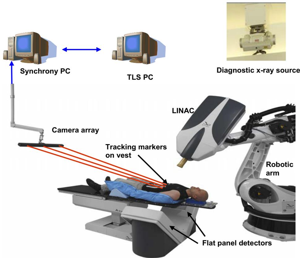
Fig. 1. Main components of the CyberKnife Robotic Radiosurgery System with the Synchrony Respiratory Tracking System are: (1) compact 6-MV X-band LINAC mounted to robotic arm; (2) two orthogonal flat-panel x-ray detectors positioned perpendicular to diagnostic x-ray sources mounted to ceiling; (3) Synchrony tracking vest with LED markers attached; (4) camera array that holds 3 CCD cameras; (5) Synchrony and Target Locating Computers. Image used with permission from Accuray Incorporated.
