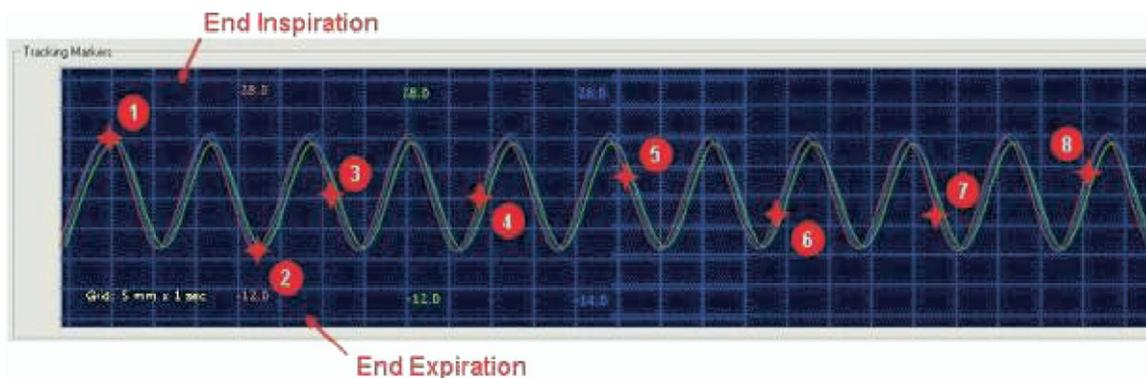
Fig. 3. Patient's breathing cycle as displayed on Synchrony PC monitor in real-time during treatment. To build a reliable correspondence model, 8 diagnostic x-ray images are taken at different phases of respiratory cycle. Four images are taken during inspiratory phase and another 4 during expiratory phase. Image used with permission from Accuray Incorporated.
