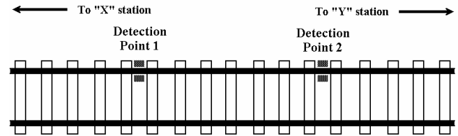
Fig. 8: Ubication of the coils in the rail line
