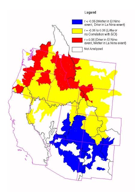
Figure 33: Correlation Map of the Southern Oscillation Index with spring and summer volume runoff
