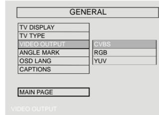
There are three video output choices: Use the CVBS output if the S-Video output jack has been selected; use the RGB output if the RGB output jack has been selected; or use the YUV output if the component output jack has been selected.
