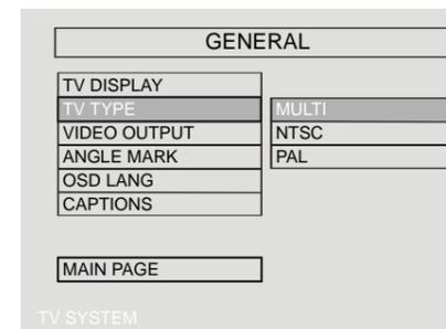
This Norcent DVD player supports output of various systems, including auto, NTSC, and PAL. If the TV set has only NTSC or PAL systems, the picture will blink and become colorless when the wrong system is selected. If this occurs, press the N/P key on the remote control to return to the normal screen. Remember to always select the correct system.
