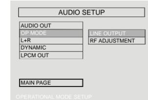
Both of the line output and RF adjustment options are applicable in all conditions. Due to its suitability and convenience in most cases, line output is used. In some conditions, for instance when headphones are used, the RF mode may be used.
