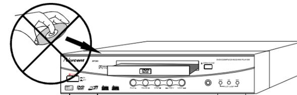
It is possible to damage a disc if it is not placed correctly on the guides in the disc tray. This may also cause the DVD player to malfunction. Do not force or place anything other than a 5 inch DVD or CD onto the disc tray.
