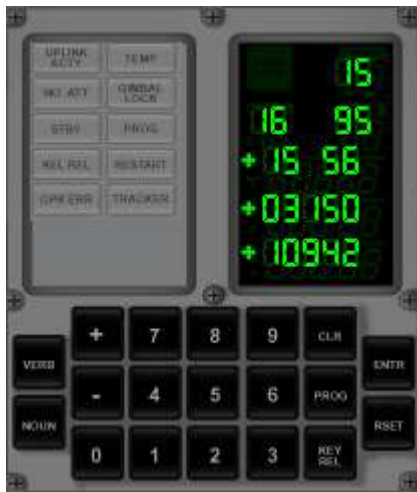
Illustration 7DSKY showing time to burn, remaining DV, & cutoff velocity
