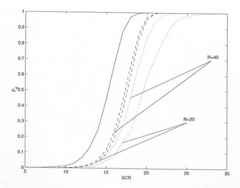
Figure 2.  $P_d$  versus SCR of the receiver (15) (dashed curve), (17) (dotted curve), and asymptotic performance  $N=\infty$  (solid curve), for  $P_{fa}=10^{-4}$ ,  $f_d=0.03$ , H=10, M=3,  $M_0=6$ , and N as a parameter.
