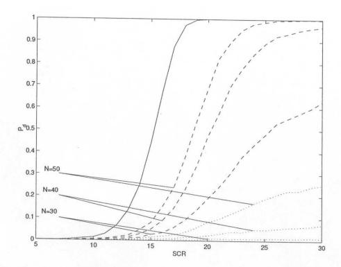
Figure 3c.  $P_d$  versus SCR of the receiver (25) (dashed curve), (27) (dotted curve), and asymptotic performance  $N=\infty$  (solid curve), for  $P_{fa}=10^{-4}$ ,  $f_d=0.03$ , H=10, M=3,  $M_0=6$ , target model  $M_3$ , and N as a parameter.
