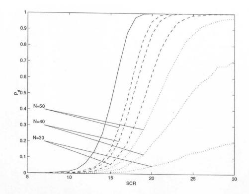
Figure 3b.  $P_d$  versus SCR of the receiver (25) (dashed curve), (27) (dotted curve), and asymptotic performance  $N=\infty$  (solid curve), for  $P_{fa}=10^{-4}$ ,  $f_d=0.03$ , H=10, M=3,  $M_0=6$ , target model  $M_2$ , and N as a parameter.
