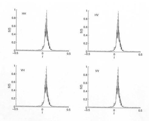
Figure 1. Power Spectral Density of the returns from the 13-th range cell versus the normalized frequency f. Model-based PSD estimates (dashed curves), non-parametric PSD estimates (solid curves).
