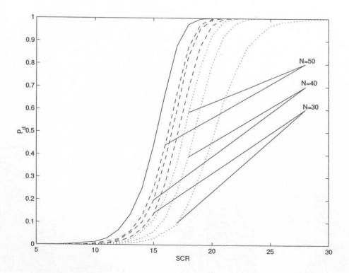
Figure 3a.  $P_d$  versus SCR of the receiver (25) (dashed curve), (27) (dotted curve), and asymptotic performance  $N=\infty$  (solid curve), for  $P_{fa}=10^{-4}$ ,  $f_d=0.03$ , H=10, M=3,  $M_0=6$ , target model  $M_1$ , and N as a parameter.
