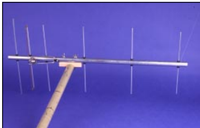
Fig 7—70-cm Yagi mounted to a 1/4-inch boom.
