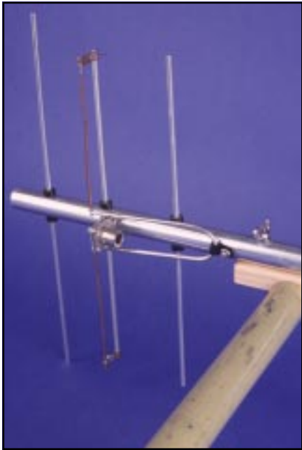
Fig 8—Yagi showing reflector, driven element and first director.
