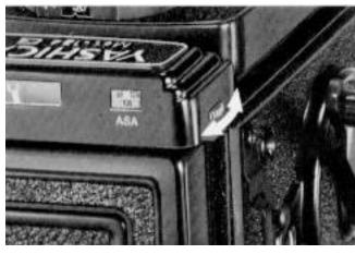
\* When the camera is to be left unused, fold the focusing hood. This will switch off the meter and prevent draining of battery power.
