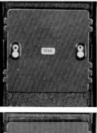
When loading a 120 film (12 exposures), hold the back cover with both hands and slide the Film Pressure Plate with your thumbs until it clicks into position and the sign 12 EX. (in green) appears in the window in the middle of the plate. When loading a 220 film (24 exposures) hold the back cover with both hands and slide the Film Pressure Plate with your thumbs until it clicks into position and the sign 24 EX. (in red) appears in the window in the middle of the plate.
