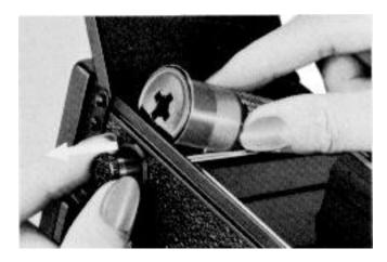
\* - To minimize the trouble in loading your next film, it is advisable to take out the empty spool from the lower film chamber and to set it in the upper chamber immediately after unloading the exposed film.
