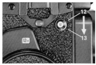
**OR** - When the figure "24" appears in the exposure counter window, it signifies that the full length of the film has been exposed. Another wind of the crank-handle will bring out the (circle?) mark in the window, but continue winding until the crankhandle turns freely without tension.
