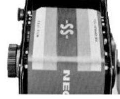
**OR** - Continue winding the film until the "start" mark on the film leader paper lines up with the RED triangular "start" mark for 220 film.
