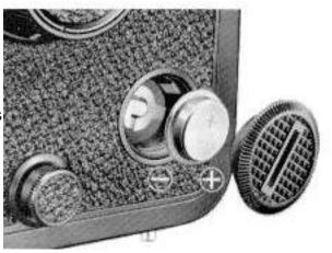
2 - Install a 1.3 V mercury battery to power the exposure meter, as illustrated.
