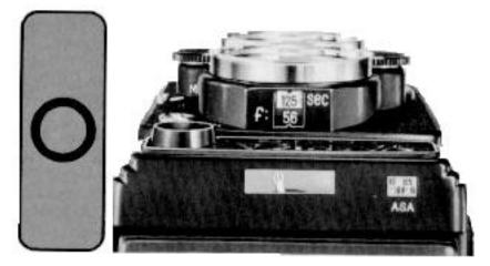
\* If the yellow follower needle fails to align with the meter pointer, alter the shutter speed setting by turning the Shutter Speed Control Dial in either direction. If the two needles fail to match even when both the shutter speed and aperture settings are changed, it means that correct exposure cannot be obtained under the prevailing light condition.
