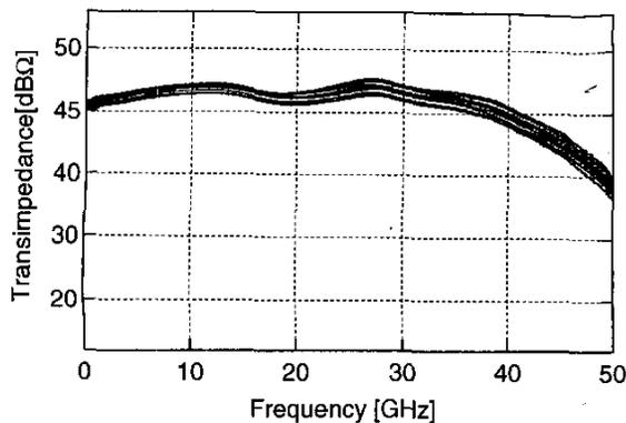
Fig. 10 Measured transimpedance of 15 representative TIAs.
