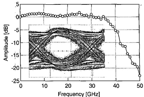
Fig. 11 Photoreceiver transfer characteristic and eye diagram.
