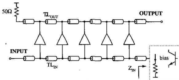
Fig. 4. Schematic diagram of the distributed TIA.
