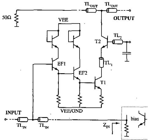
Fig. 6. Schematic of the gain cell.
