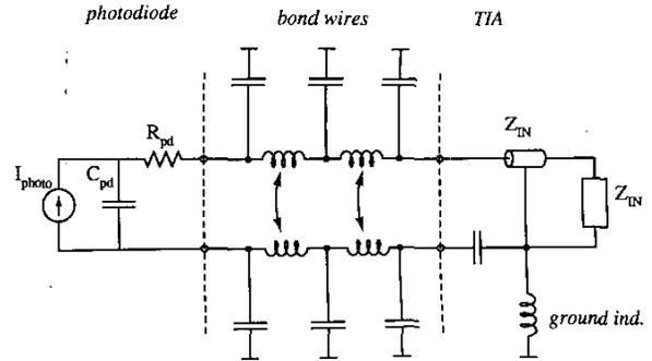
Fig. 5. Equivalent circuit model for the TIA input.
