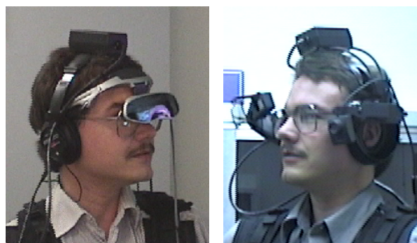
Figure 4. Head-worn displays: left: SONY Glasstron display with headphones and Cybertrack on top. Right: Monocular display and head set from Xybernaut. A camera is attached on the left head side.
