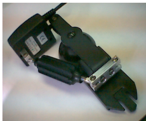
Figure 3. Retrofit Xybernaut camera for more stable orientation fixation.
